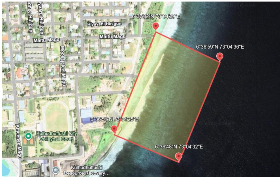
Figure 0-1 Area for preliminary bathymetric survey (21.77 acres)
